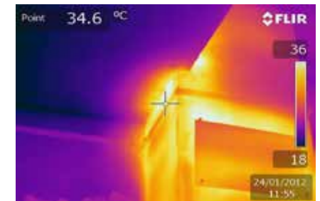
Hot water pipes hidden behind the wall are leaking. In this case visual signs of water leakage are present. The thermal imaging camera helps to pinpoint the leak location.
