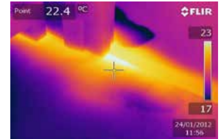
The thermal image clearly shows that an underfloor hot water pipe is leaking.
