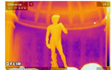
This thermal image reveals the underlying texture of the walls and pillars of the apse.
