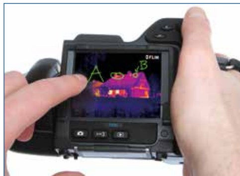
Thermal image of the same building, now using the MSX-setting. Note that more details are visible, making it easy to locate ventilation grids and see brick structure.
