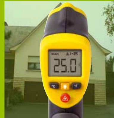
IR thermometer, temperature measurement in one spot
