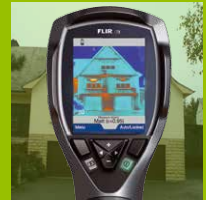
FLIR i3, temperature in 3,600 spots
