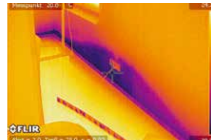
This case of water damage clearly shows the advantage of the Picture-in-picture feature, since the client can quite easily see where this thermal image is located, while this would be more difficult with only the thermal image.
