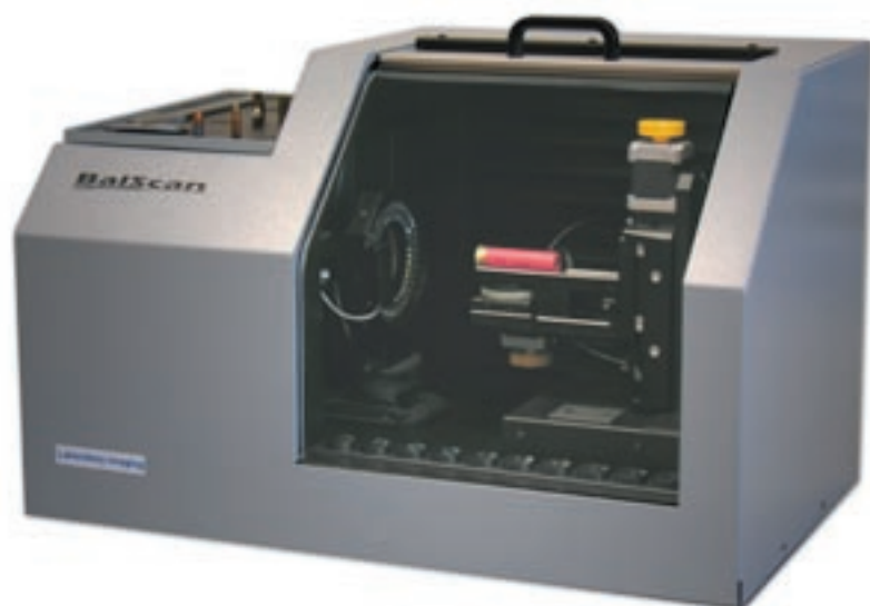
LEFT: The current fully functional prototype of LUCIA BalScan developed at Laboratory Imaging. The device enables a comfortable operation of bullets and cartridge cases.
