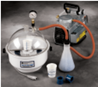
Cast N' Vac 1000 Vacuum Impregnation System for impregnation of porous specimens.
