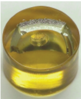
Acetabular Cup mounted in EpoHeat® Epoxy.
