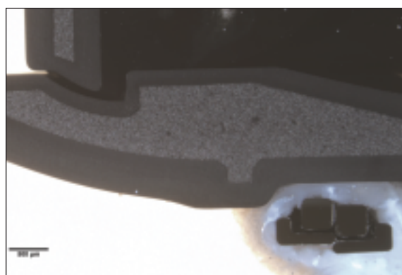
Pryolitic heart valve cross-section.
