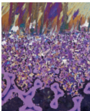
Microstructure of Acetabular Cup, Ti-6Al-4V Substrate with CP Ti Powder.
