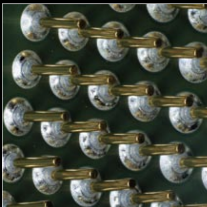
PGA tilt observation (Ring illumination)
