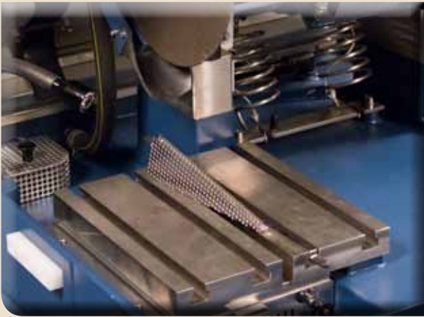
Helpful and convenient, removable basket helps catch small parts when cutting.
