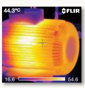
Internal winding problems and other defaults in motors and mechanical systems become clearly visible on the LCD touch screen of the FLIR E-Series.
