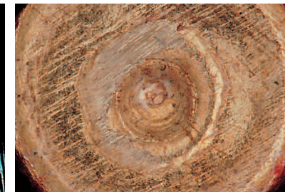
Bullet, impression after use, at 50x
