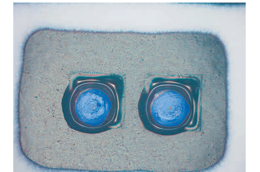
0402 laminated ceramic pad at 200x
