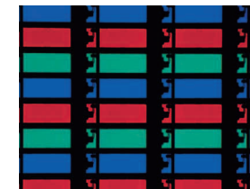
LCD panel at 700x [Backlighting]
