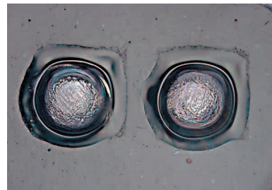
0402 laminated ceramic pad at 200x
