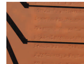
Indentations of LCD conduction poles at 200x [Differential interference]
