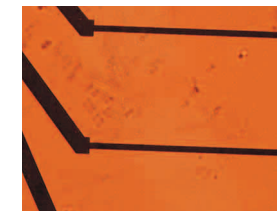
Indentations of LCD conduction poles at 200x [Bright field lighting]
