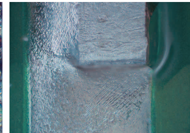
Solder fillet of a QFP contact at 300x
