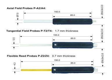
The following axial field, tangential field and flexible reed probes are available for the MP-1000 and MP-2000 Field Meters:
