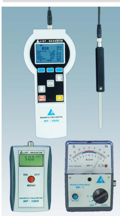
Magnetic field meters are used for the precise measurement of all kinds of magnetic field (steady and alternating fields, as well as pulsed fields).
