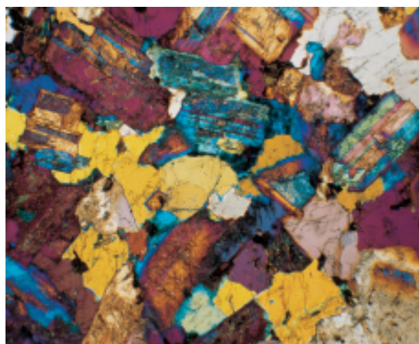
Granite thin section, under cross-polarized light (first order red plate), ~127x. Transmitted light.
