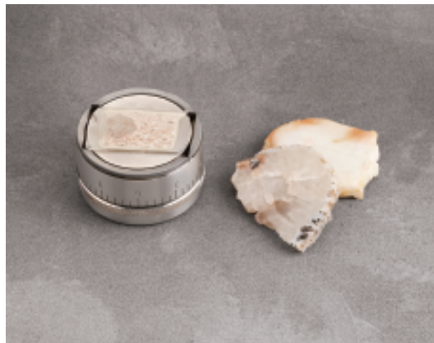
Histologic Precision Grinding Fixture 60-8087 will hold a 27 x 46mm (1 x 1.8") glass slide and is ideal for precise material removal.
