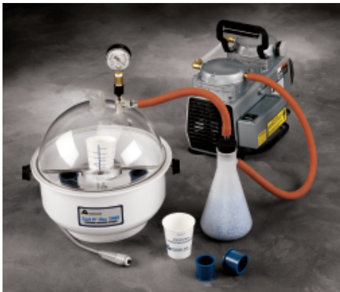
The 20-1382 Cast N' Vac 1000 is ideal for impregnating geological samples with a suitable bonding material that fills pores, cracks, and retards sample fracturing or plucking.
