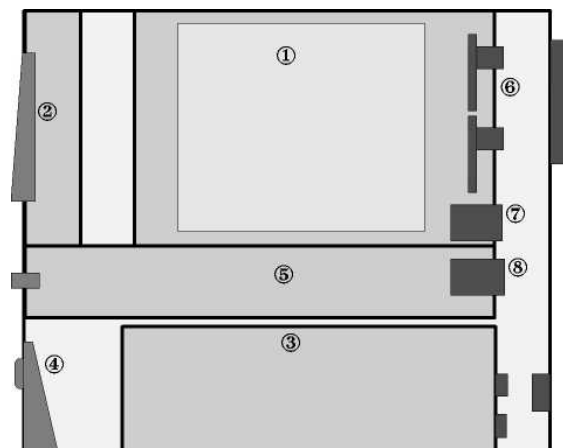
Fig. 16: Compact housing 12 height units, electronic test unit, integrated PC, schematic
