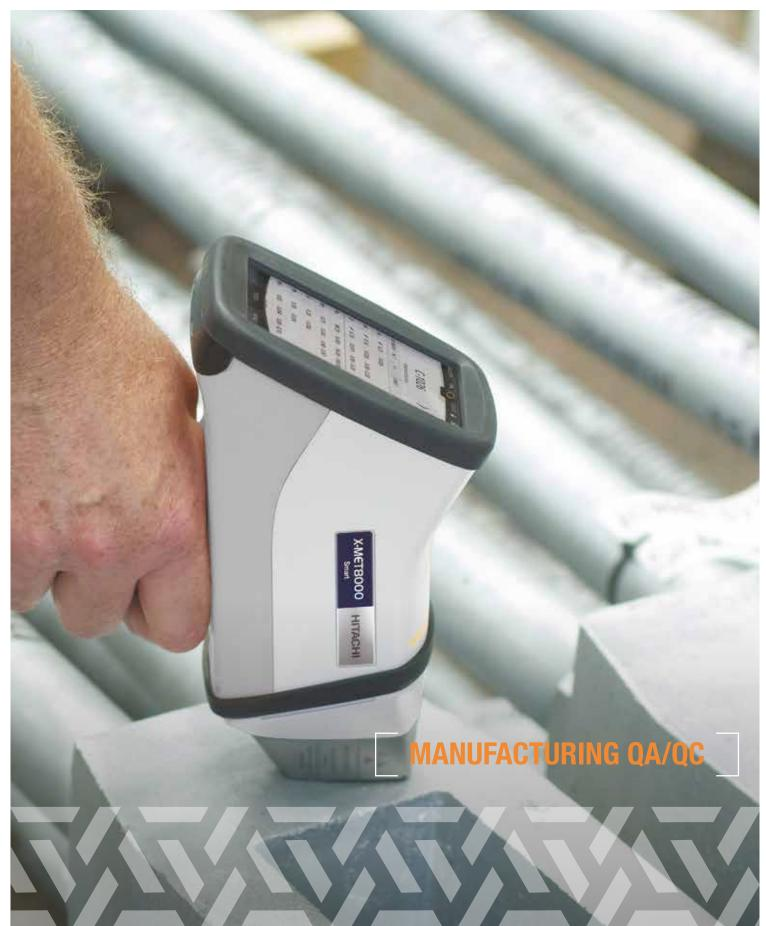
The X-MET8000 is a handheld X-ray fluorescence (XRF) analyser that delivers fast, non-destructive analysis and accurate grade identification for manufacturing quality control and assurance. The combination of a high performance X-ray tube and large area silicon-drift detector (SDD) delivers the performance required for even the most demanding QA/QC applications. With X-MET8000 you get laboratory quality results in seconds, reducing testing costs and time.
