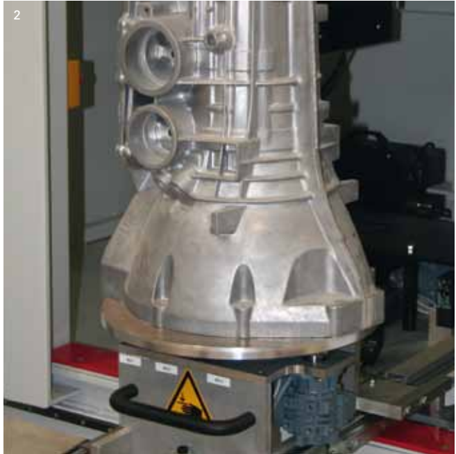
1 Casting on turntable 2 Loading and unloading outside of the cabinet
