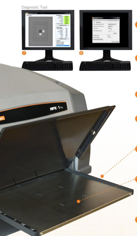
**System Status** - Diagnostic Tool (optional accessory) allows user to check system status per ASTM E2445.
