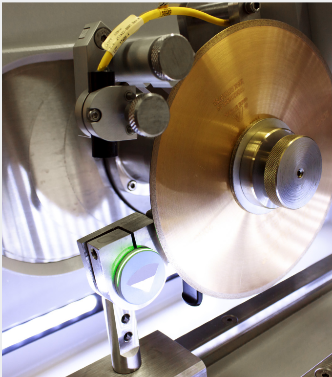
Users can see exactly where the cut will travel along the sample with the precision laser.
