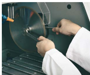
Easy Exchange of Cut Off Wheel
