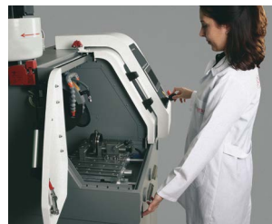
Two Hand Control For Safety Operation
