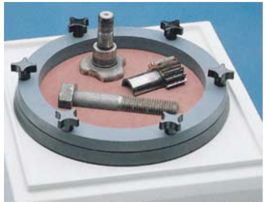
Large unmounted specimens may be polished with ease. Once loaded, specimens require little operator attention.
